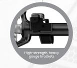
Axle tubes: 3½" outside diameter/.370" wall thickness
