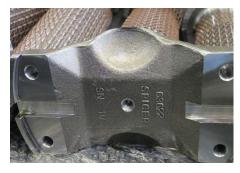
Now, with laser marking, Dana will have better control over font size and type used to mark products, delivering a crisper appearance of the Spicer name through a more reliable and constant process.
