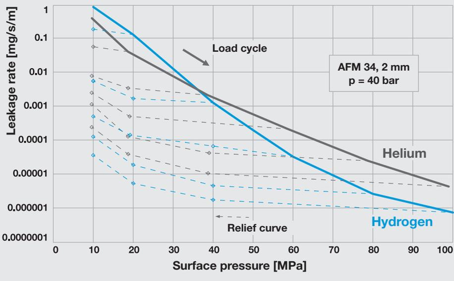
**▲ Diagram 1:** AFM 34 leakage rate at surface pressure as per EN 13555. Comparison of test media helium and hydrogen at 40 bar.
